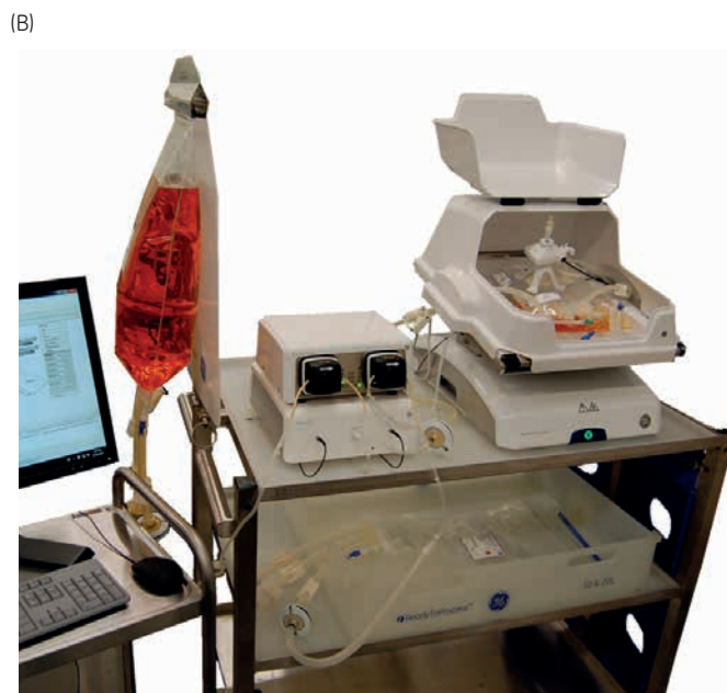
Fig 1. Vials from a high-density cell bank can be used for direct inoculation of a small bioreactor culture, eliminating the need for shake flask operations in the immediate post-thaw expansion phase. The use of perfusion in the bioreactor stage allows cells to stay in exponential growth phase throughout the entire culture, for high final viable cell density and cell viability. By such a procedure, an N-1 culture at 10 L scale can be used to seed a production culture with a final volume of 2000 L.
